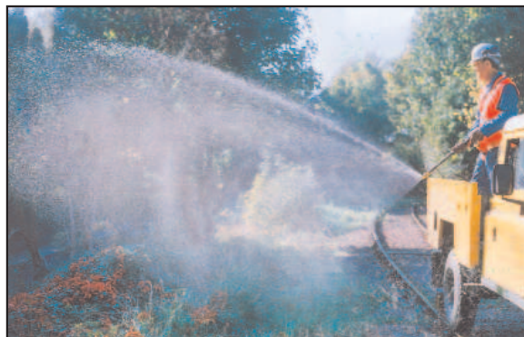
(Above) The operator riding in the trailer can spray selectively using a hand-held lance. (Below) Similar procedure is possible using the Land Rover unit. (Bottom right) Fixed off-track spraying can cover a five-metre swathe.
