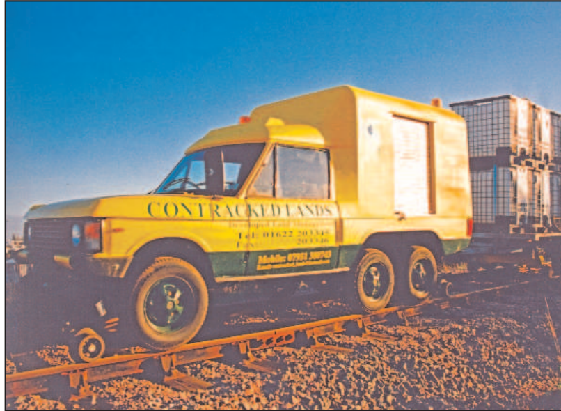
The road/rail Range Rover can spray up to 20 miles of track with a five-metre swathe when the trailer tanks are employed to supplement the unit's basic water capacity. Contrackeds Lands converted this vehicle from a fire support unit.
